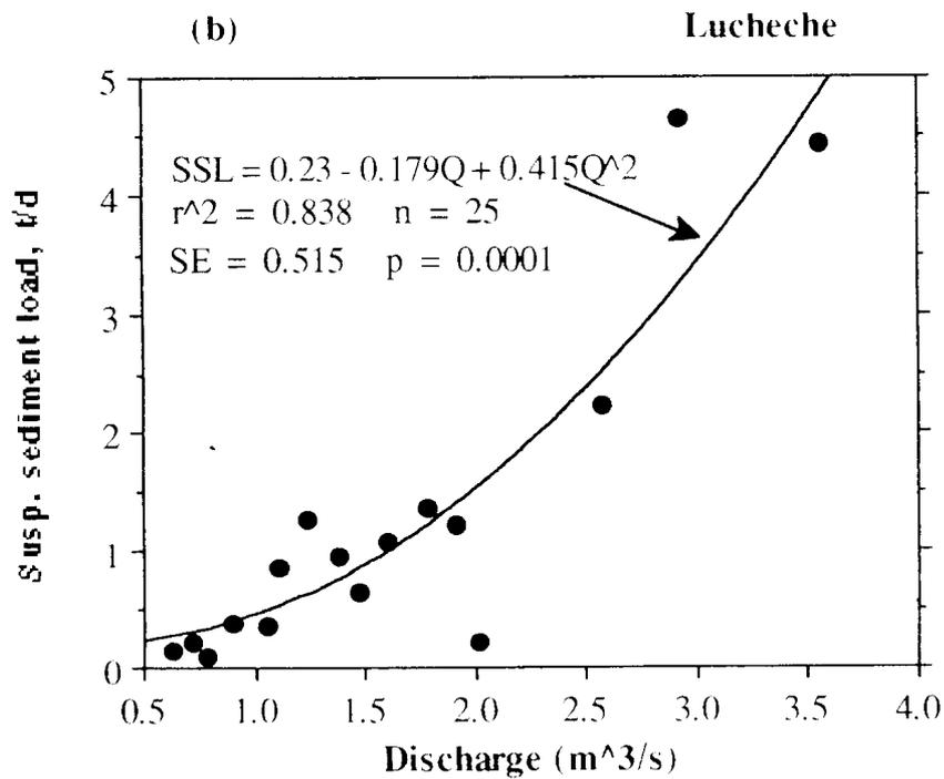
Figure 2. Rating curves for Lucheche River at Kawe Village (a) discharge, (b) sediment load, September 1998 - December, 1999.
