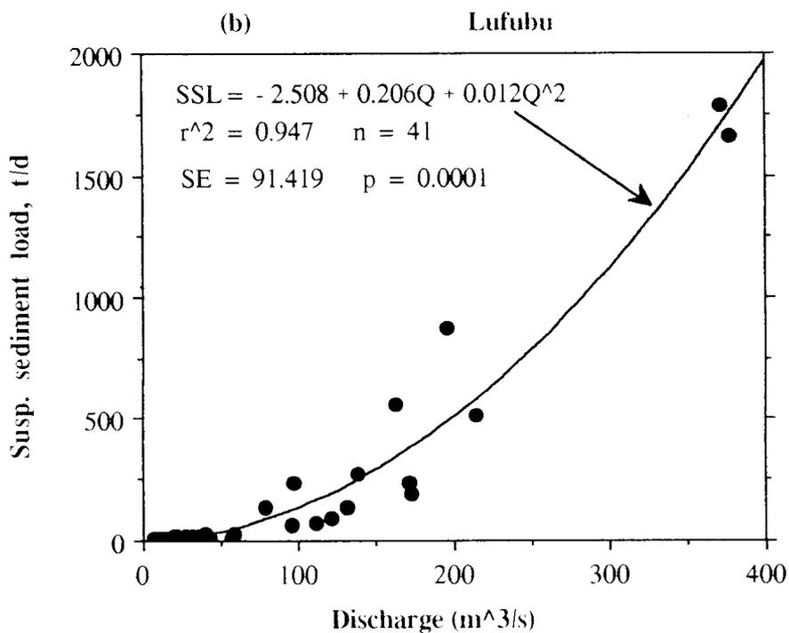
Figure 6. Rating curves for Lufubu River near Kabyolwe Village (a) discharge, (b) sediment load, September 1998 - December, 1999.
