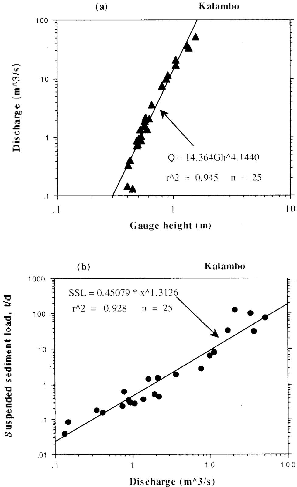
Figure 3. Rating curves for Kalambo River at Kalambo Village (a) discharge, (b) sediment load, September 1998 - December, 1999.
