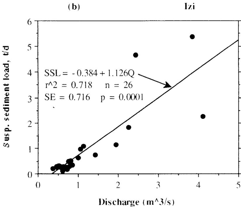
Figure 4. Rating curves for Izi River at Mbete Village (a) discharge, (b) sediment load, September 1998 - December, 1999.
