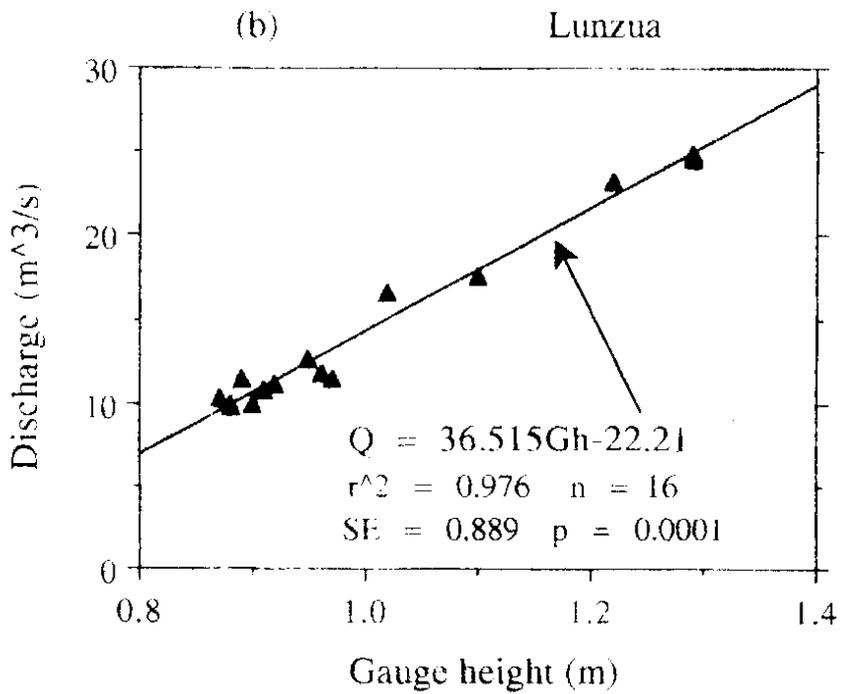
Figure 14. Discharge rating curves for (a) Izi River at Mbete Village, and (b) Lunzua River at Simumbele Village, September 1998 - May, 1999.
